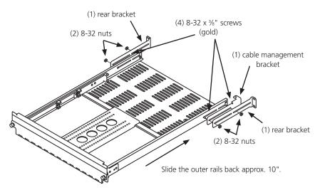
Figure 4. Attaching the rear bracket.
